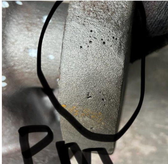
Gambar 4. Defect porositas mikro
